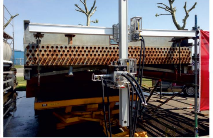
Cleaning of inside bundles and outside finned pipes. The cleaning system is easily adapted on the finned tubes surface by using special design coupling devices.
